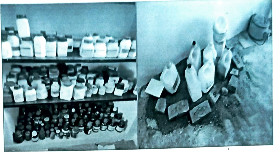
Fig.2: Storage of Chemicals /Salts /Acids& Laboratory Equipments (Rack & Sand Bed)
